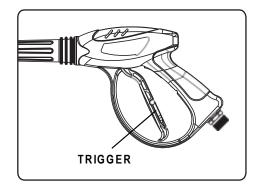
AN WARNING! Kickback forces result from pressing the trigger! Therefore, always hold the spray gun with both hands! Pay attention to safe posture! Improper handling may result in injury!
